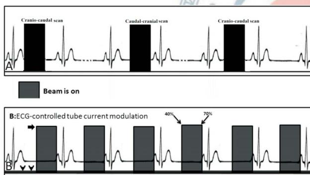
**Figure 2.** Model shows ECG gating in Flash vs. RGH: (A) in flash high pitch gating: the X-ray is on during the scan only (single heart beat) in cranio-caudal direction, caudal-cranial and cranio-caudal scan. (B) in RGH scan: X-ray is on throughout the cardiac cycle with maximum intensity between 40% and 70% of RR interval (black arrow), while it drops to 5% at the rest of RR (arrow head).
