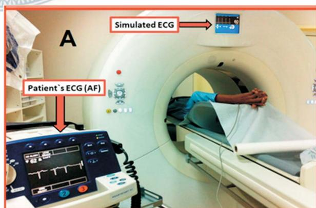
**Figure 1.** Patient position and monitoring during NGTF scan. The scan considered non gated scan as it triggered by a built-in simulated ECG but not the patient's ECG.
